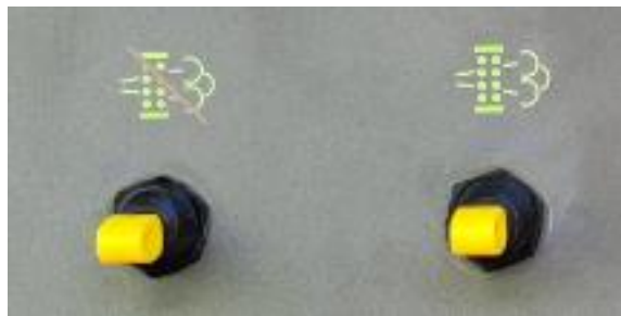
Fig.5-17 DPF regeneration prohibition button and regeneration button
