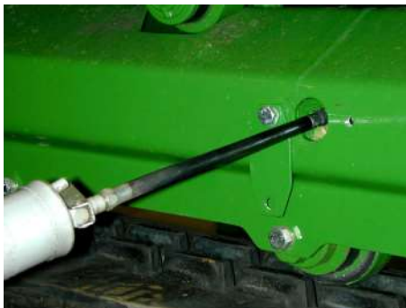
Fig. 67 Grease gun on grease nipple for the tension roller
