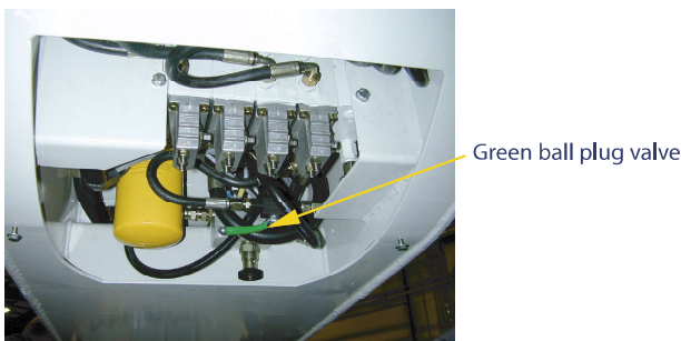
Fig 45a Green ball plug valve for emergency lowering
