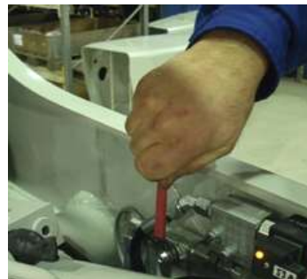
Fig. 36a ball valve emergency basket leveling.
