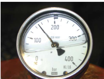
Fig. 68a Pressure gauge on Grease gun
