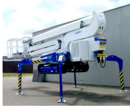
Fig. 58 Platform lifted by the outriggers
